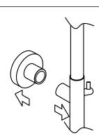
Step 6 Remove the riser and the mounting piece.
